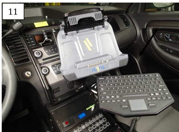
Ford Interceptor Sedan application DS-PAN-701, C-DMM-122, C-MM-201, C-MM-301 C-MD-204, C-KBM-101 and C-VS-1508-INSE
