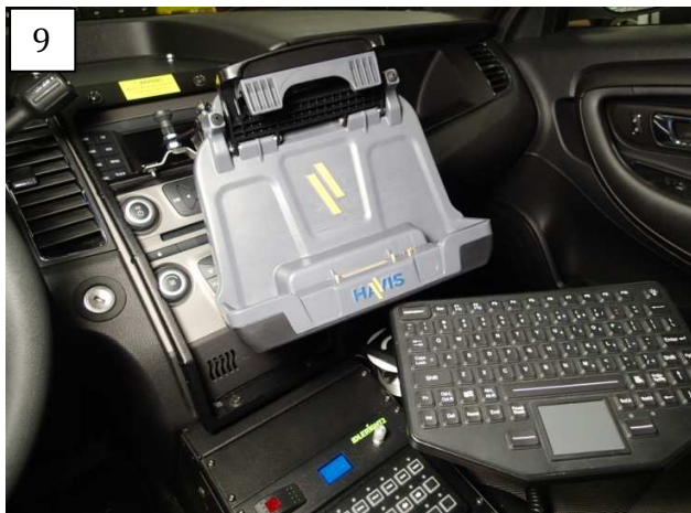
Ford Interceptor Sedan application DS-PAN-701, C-DMM-122 (with New Vesa 75), C-MD-204, C-KBM-101 and C-VS-1508-INSE
